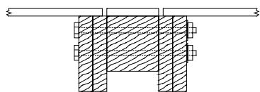
Use feature boards to break up the deck into "manageable" sections of shorter lengths. The structure must be modified to support the feature board while also supporting the ends of the deck boards running up to it. To do this, a wood 6x6 is installed directly below the feature board and two joists are installed on either side of the 6x6. These are all joined together using bolts with nuts and washers (see end-view illustration).
