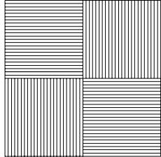
The layout of the deck can be designed in a way to break a very large (i.e. 24' x 24') deck into quadrants of alternating board directions (see top-view illustration).
